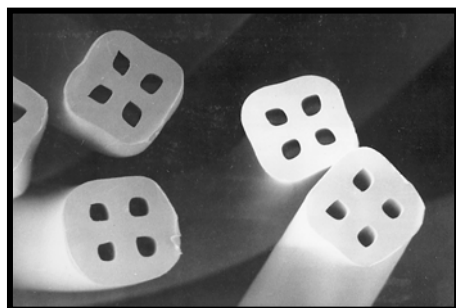
Nylon Type 6.6 hollow core and round cross-sections
