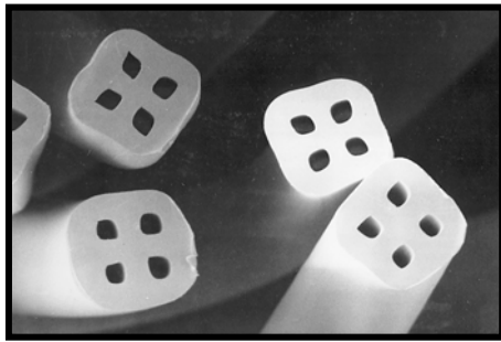
Nylon Type 6.6 hollow core and round cross-sections
