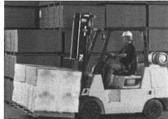
Figure 14. Operator traveling with load lowered.
