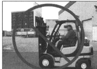
Figure 15. Do not travel with the load elevated.
