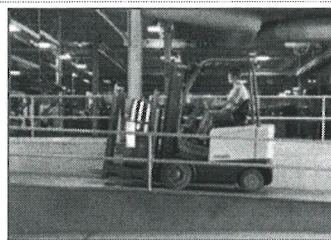
Figure 12. Drive loaded trucks forward going up a ramp.
