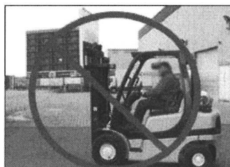
Figure 15. Do not travel with the load elevated.
