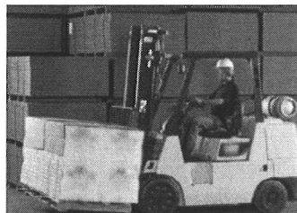
Figure 14. Operator traveling with load lowered.
