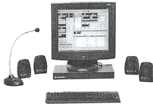
Figure 1-2: MCC 7500 Operator Position.
