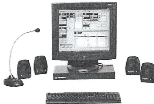
Figure 1-2: MCC 7500 Operator Position.
